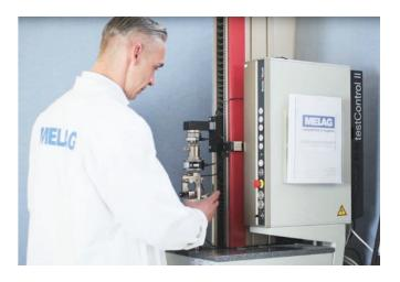
In order to validate packaging processes and to evaluate the performance of sealing devices, hygiene experts strongly recommend the seal seam stability test as an annual routine check.
