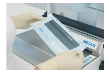
The daily MELAcontrol Seal Check verifies the quality of the seal seam in accordance with DIN EN ISO 11607-2.
