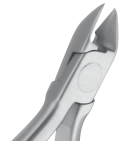
Slim Micro Cutter 678-500 Wire size: \leq .008'' to .012'' The slender tip allows for easier access when removing elastics. The face of the cutter has been scooped out and reduced by 13% as compared to our original 678-110 to enhance visibility.
