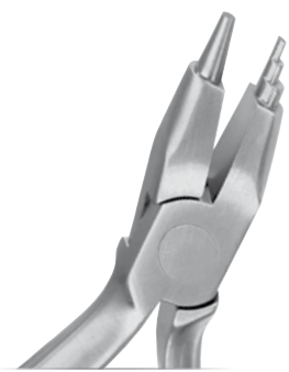
Marcotte Looping Pliers 678-316 Wire size: \leq .022'' \times .025'' (.56 mm x .64 mm) For precise forming of helical loops and T loops. No right angles. Prevents stress fracture of wires.
