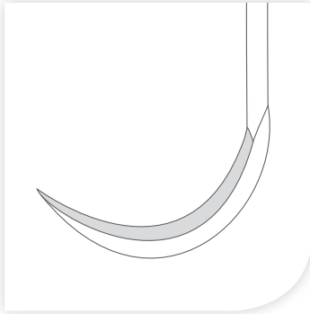
THE CURVED SICKLE SCALER Two cutting edges on a curved blade that end in a sharp point.
